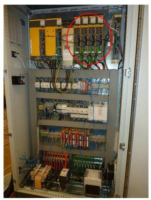
In top side of every servo amplifier, read Fanuc label to know the model of servo amplifier.
