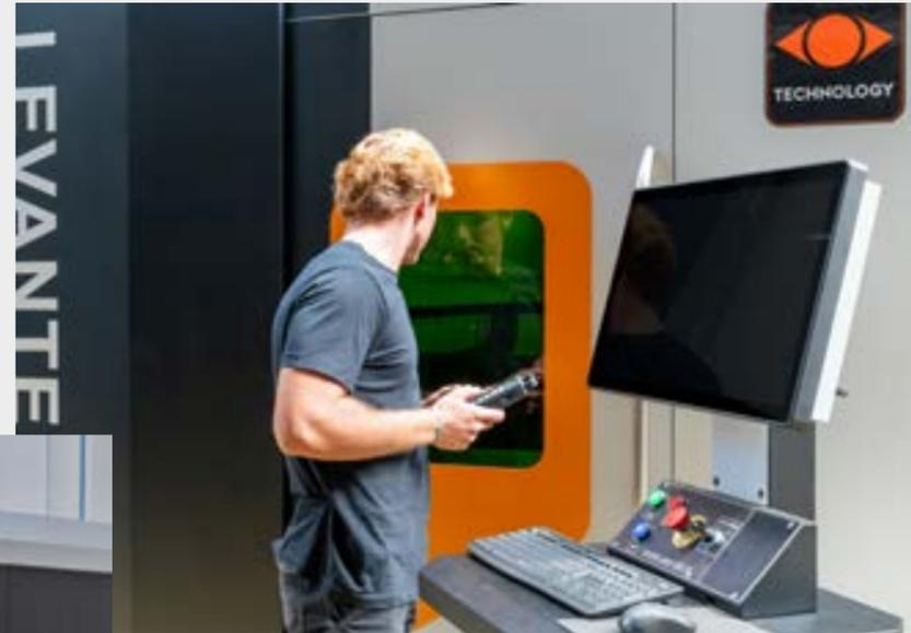
The machine's console is designed to make the operator feel comfortable right from the start. Moreover, being separate from the machine allows for a broader view of both sides.
